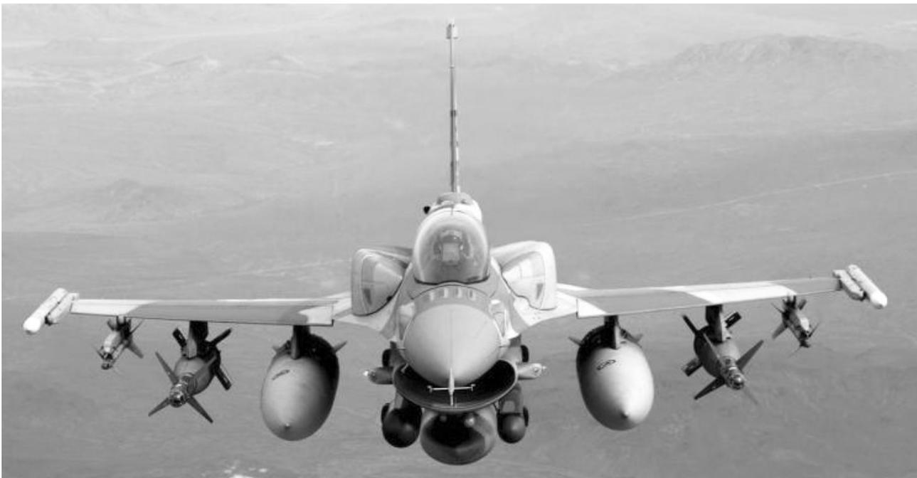
*F-16I. Note the conformal tanks at the wing roots.*
